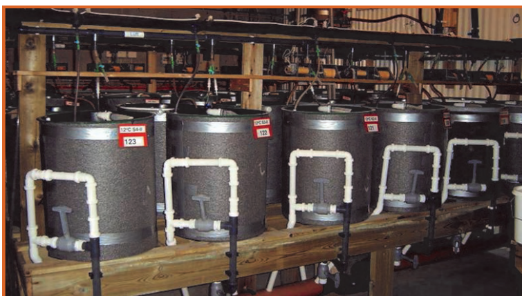
Figure 1. Experimental start feeding units with water and air temperature control.
